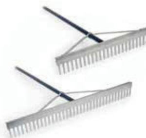
Use for: Ground Raking, smoothing, leveling, spreading, seeding & leaf clean-up. 66" long handle with rubber tip, rounded tips on teeth for lawns, beveled back-edge of blade for smooth grading, one piece heavy-duty brace riveted to rake head.
