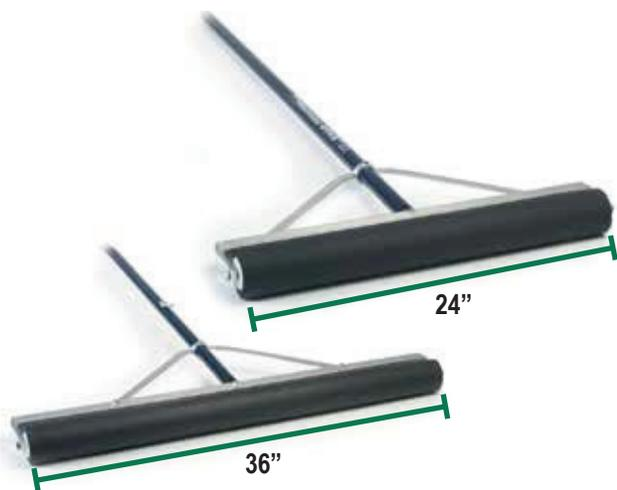
High strength double-ribbed aluminum channel, Corrosion resistant material. Durable closed cell foam rubber roller and completely watertight assembly. Roller hub made of industrial grade bearing material. Stainless Steel axle. Solid reinforced end bracket. 66" handle
